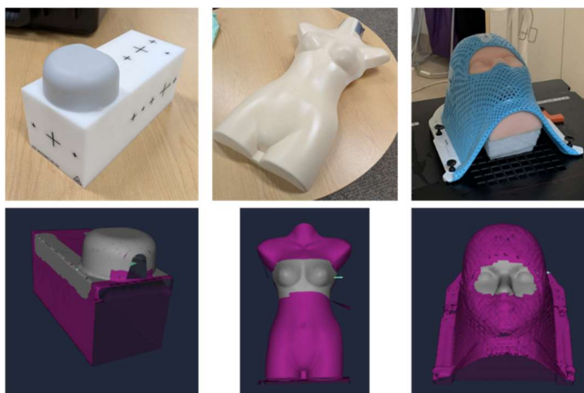
Figure 3 – The modified MultiMet-WL (left), torso (centre), immobilised head (right) phantoms used for commissioning tests.
